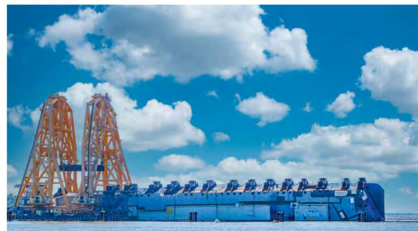
RIGHT Instability caused the Golden Ray car carrier to capsize in 2019. In 2021, the salvage operation was estimated at US\$842 million. It involved cutting the vessel into pieces using a floating crane.
