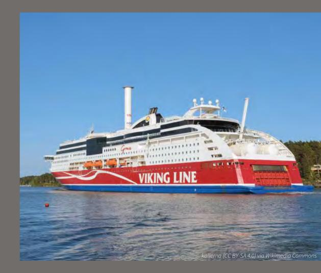
**ABOVE** The ferry Viking Grace, classed by LR, was the first passenger ship of its size to run on completely sulphur-free liquefied natural gas (LNG) when it came into service in 2013. In 2018, LR also approved the safety of the installation of a rotor sail, making it the first passenger ship in the world equipped with this type of sail to use wind power.
