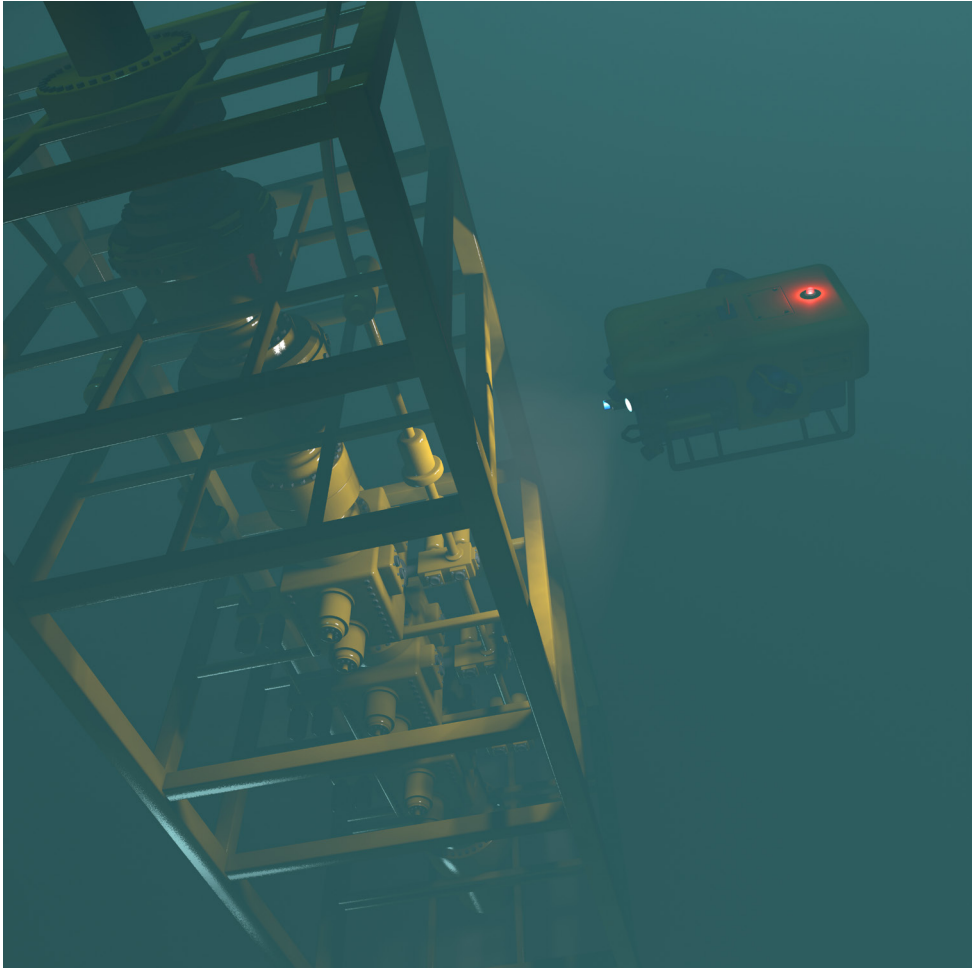
An autonomous underwater vehicle inspecting underwater oil and gas equipment. RAS are already being used to enhance safety and these capabilities might grow.
