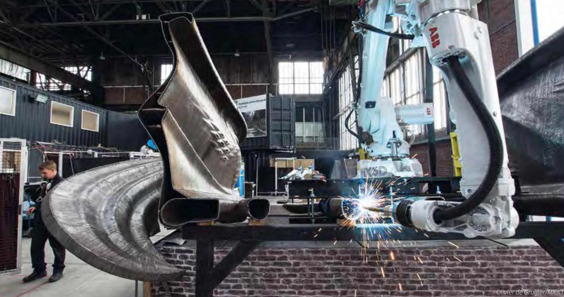
**LEFT** The metal-printing process used by MX3D is radically faster than any previous 3D-printing technology, but it cannot yet compete commercially with standard materials of construction. The bridge demonstrates that traditional elements can be combined with 3D-printed parts for bigger developments.
