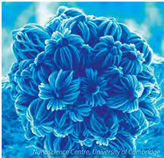
**LEFT** Nano flower bouquet, a three-dimensional nanostructure grown by controlled nucleation of silicon carbide nanowires.
