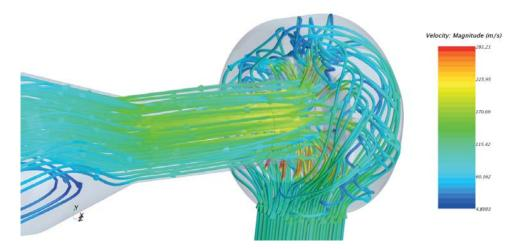
Figure 3: The image shows tracked particle velocities as gas carrying sand particles move from below up through the choke (a control on liquid flow) and on in to production system. The green represents higher velocities and the blue lower velocities. This modelling using CFD enables erosion risks in wells and production systems to be identified. Figure courtesy of LR Senergy.
