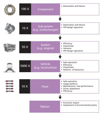
Figure 5: Data can be collected and analysed at multiple scales within a rail fleet. Credit: Richard Stobart.
