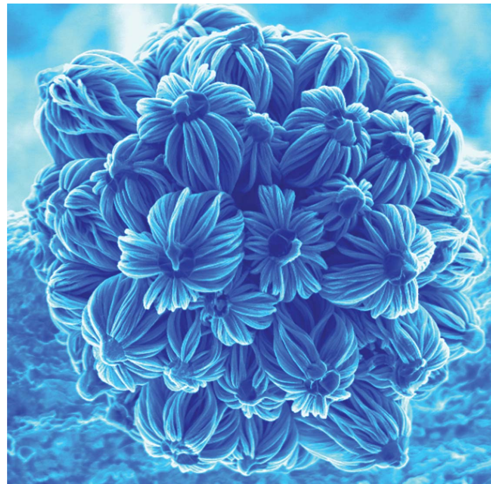
Nano flower bouquet, three-dimensional nanostructure grown by controlled nucleation of silicon carbide nanowires
