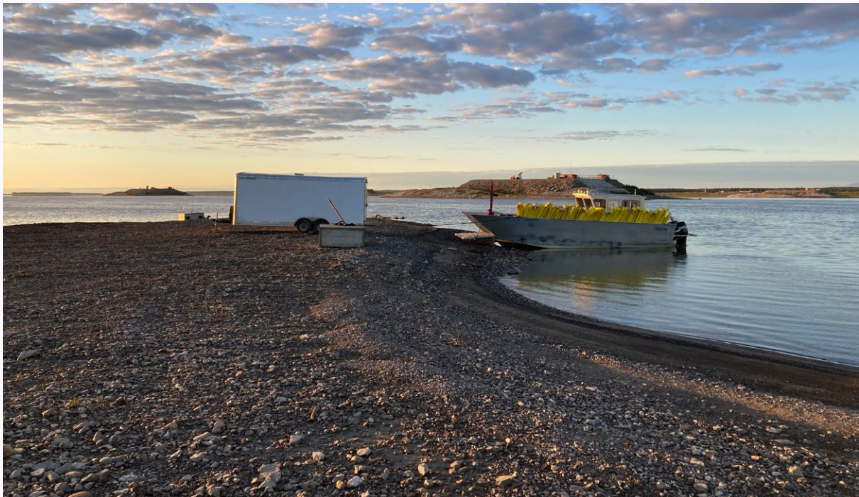
Figure 5: Spill response vessel and equipment mobilisation in Arctic Canada. This vessel and trailer setup demonstrates how spill response gear can be mobilised near shorelines when road access is not available. The vessel shown is equipped with a boom, ready for deployment in Arctic conditions.
