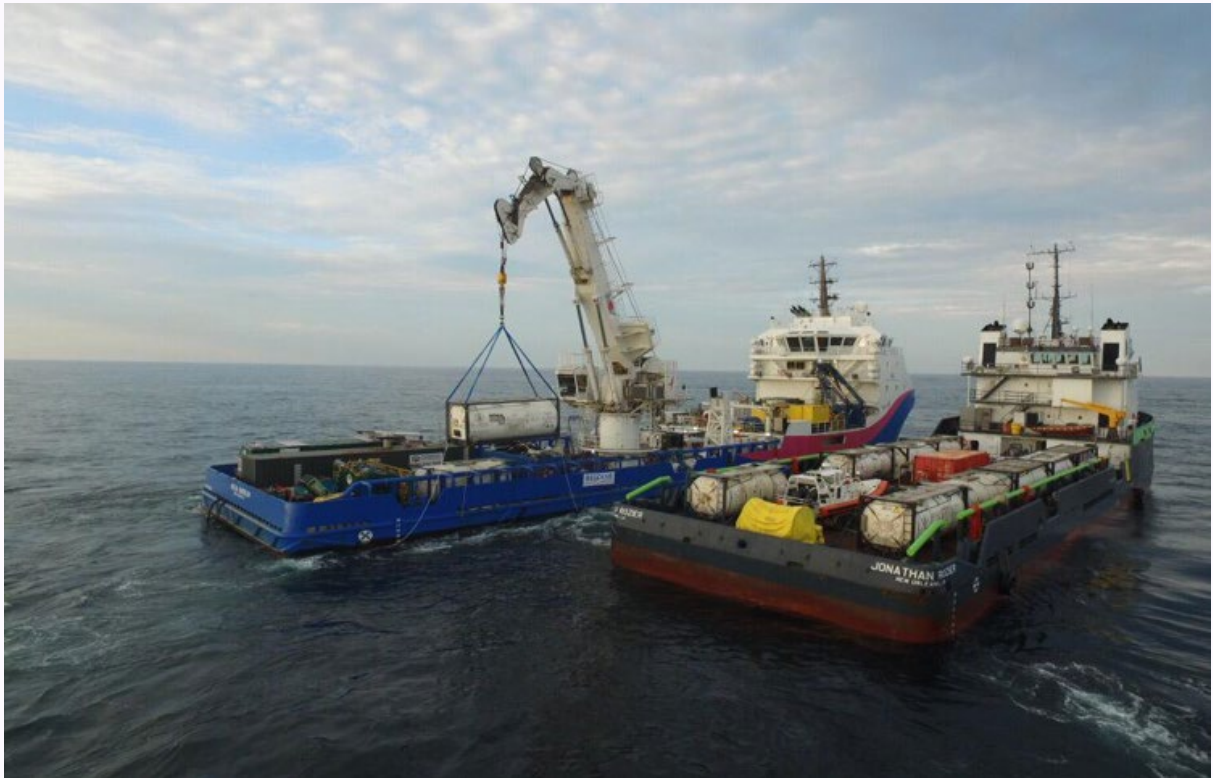
Figure 7: The successful removal of oil from the wreck of the Coimbra (a tanker sunk off New York, USA during World War II containing 1,500 tonnes of oil), conducted by Resolve Marine, required a team of 83 people and 193 dive sorties to complete the operation in approximately three months offshore.
