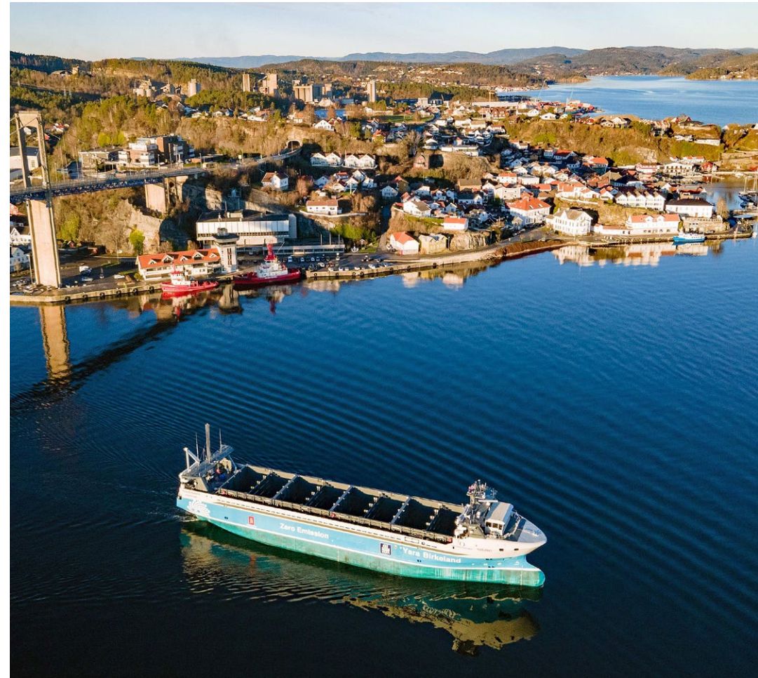
Figure 12: The first autonomous and zero-emission container ship, Yara Birkeland (source: Knut Brevik Andersen, free access granted by Yara International ASA© all rights reserved)
