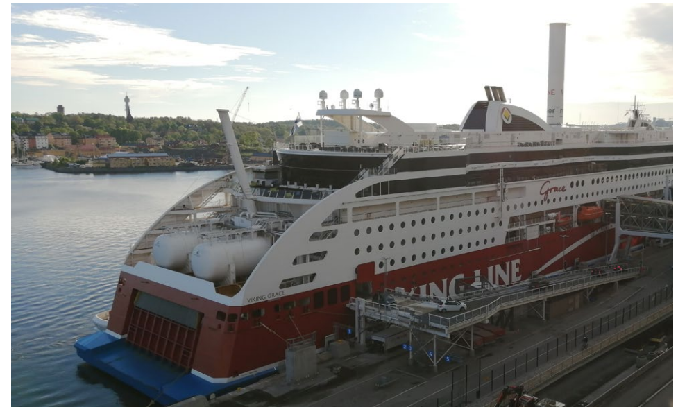
Figure 9: Viking Grace equipped with LNG fuel tanks and rotor sail in Port of Stockholm (photo taken by the authors)
