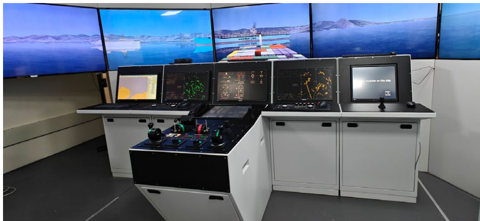
Figure 7: Bridge simulator including ECDIS from Bandari Maritime Academy, Kenya (photo taken by the authors)
